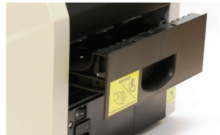
Open the rear like a drawer to get full access for cleaning and removing damaged banknotes.
