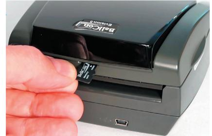
Software can be updated by inserting a standard microSD memory card in the rear side slot.
