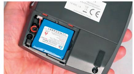
Evision 5 can be equipped with a rechargeable battery (optional).
